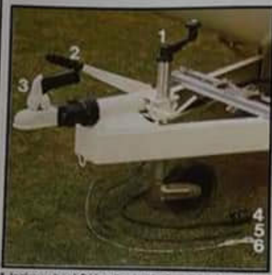
1 Jockey wheel. 2 Handbrake. 3 50mm hitch head with quick release safety lock. 4 7 pin trailer connector (electrics). 5 Refrigerator 12v feed. 6 Safety cable.
